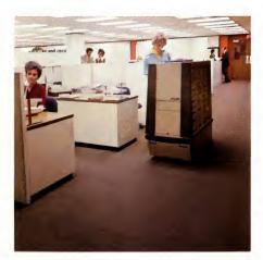
At each designated stop, incoming mail is removed from trays. Outgoing mail is placed into rear drop boxes. Inter-office mail is placed into appropriate trays and travels directly to the recipient, eliminating further sorting. After the stop interval, Mailmobile automatically resumes travel.
